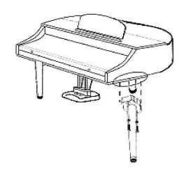
7. Using the screwdriver provided attach the headphone holder to the bottom of the piano with four machine screws into the pre-drilled holes.
