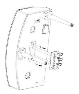
3. Attach Lyre supports to the lyre and piano body as shown. Use two lyre screws at each point shown.
